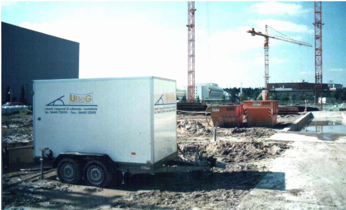
Fig. 6: Thermal Response Test equipment on site in Langen
